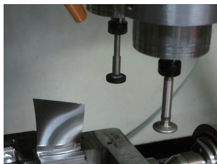
图8 超硬磨料悬臂磨削加工叶片 Fig.8 Blade in grinding utilizing super abrasive wheels
